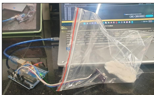
Figure 5. Detection of formalin through MS1100
