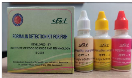
Figure 1. Bangladesh Council of Scientific and Industrial Research (BCSIR) kit for food formalin detection
